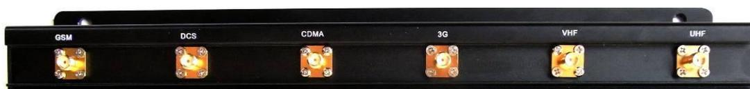
CDMA/GSM/DCS/PCS/3G/2.4G/4GWIMAX RF Output ports (connect antennas)
